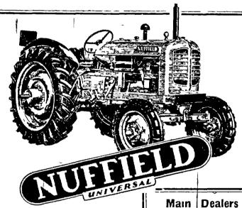
Latest and best of British tracand stockists tors the Nuffield Universal offers more advanced features greater economy and all round service than has even been com-Sherrard bined in one tractor before Delivers 38 hp pulls 4-furrow plough on medium and 3-furrow hydraulic lift and belt pulley No special implements required Diesel Model from £718 Vapourising Oil Model from £532
