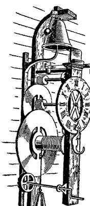
WEIGHT - DRIVEN CLOCK (15th Century) The invention of the mech anical weight-driven clock came about the fourteenth century and during the next hundred years these clocks became quite common Illustrated is the construction of an Italian weight-driven clock. It s one hand—the hour hand—was fixed, and the time was registered by the revolving of the dial.
