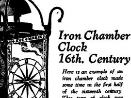
some time in the first half of the sixteenth century This type of clock was driven by weights and the wheelwork was set at right angles to the dial which told the hour There was no register for minutes.
